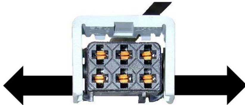
Gently pull the latch out away from the UEGO Sensor connector
